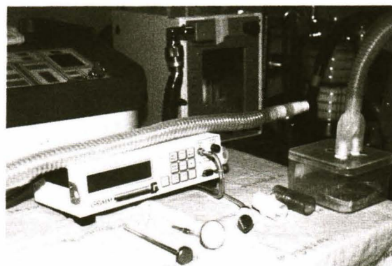
Fig. 2. Lung model machine in the center, airway passage with a box for laser evaporation on the right, laser diode portable dust monitor with adaptor and accessory on the left.
