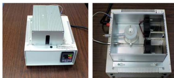
Fig. 4 In-house temperature control box with QCM detection system. The QCM sensor was inserted into the flow cell inside the temperature control box and connected with the frequency counter (17) .
