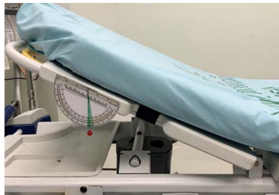
Figure 1. The tool used to measure the angle of the bed head (a small plumb attached to a protractor). The ramped zone is displayed in green (20 to 30 degrees).
