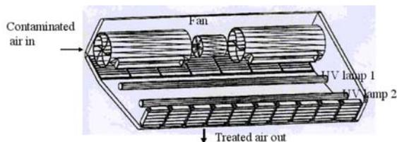
**Fig. 1** Ultraviolet germicidal irradiation (UVGI) device
