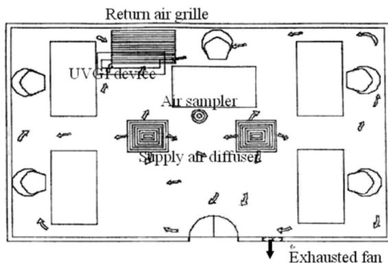
**Fig. 2** An airflow diagram within the test room
