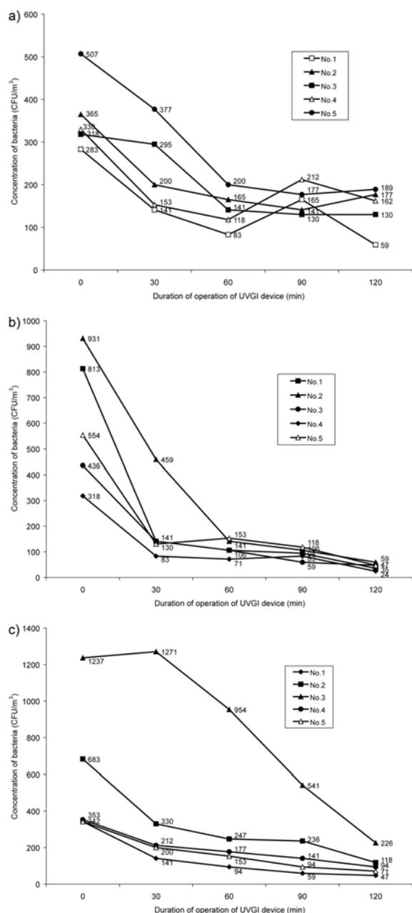
**Fig. 4** Concentrations of bacteria after operating the UVGI device at a flow rate of a) 15.7 m<sup>3</sup>/min, b) 31.6 m<sup>3</sup>/min and c) 46.1 m<sup>3</sup>/min for 30 to 120 minutes
