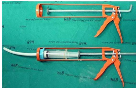
**Fig. 3** A household silicone caulking gun before and after assembly with cement cartridge and nozzle
