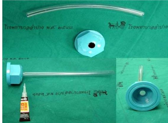
**Fig. 1** The nozzle (It is made from a 1" PVC internal threaded cap and 3/8" PVC garden hose, secured with cyanoacrylate glue)
