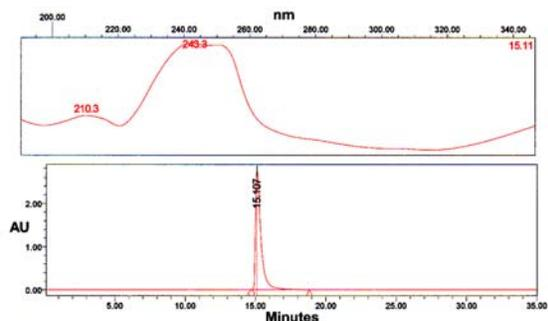
**Fig. 1** Chromatogram of barakol (25 mg) dissolved in HPLC water (1mg/ml) measured by HPLC-PDA (190-350 nm, Waters, USA) using Kromasil C8 column (250 mm x 4.6 mm ID, 5 mm particle size) and flow rate of 0.8 ml/min. The compound had a characteristic absorbance at 230 - 260 nm with the highest absorbance at 243.3 nm and the runtime of 15.107 minutes
