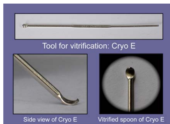
Fig. 1 Shape and all views of Cryo-E (sterilized stainless steel ear pick)
