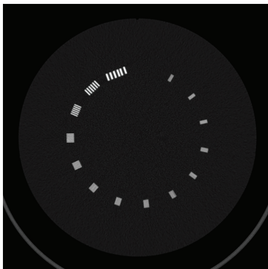
Figure 1. For spatial resolution, the investigator chose the maximal line pair (lp/cm) that was still visible as a set of separable black and white lines.
