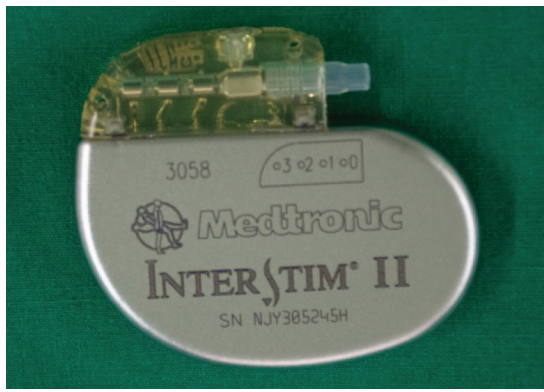
Figure 6. Stimulator (battery/impulse generator).
