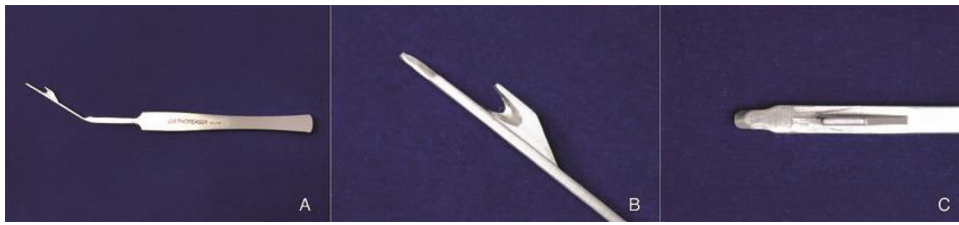
Figure 1. A side view of the newly-designed instrument (A). A side view (B) and top view (C) of the cutting part.
